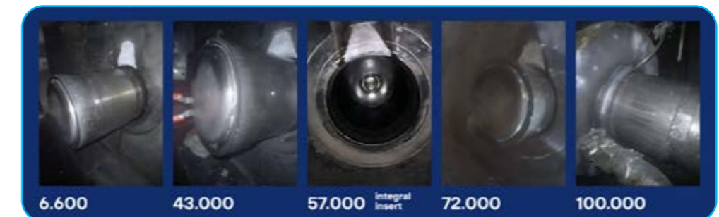
Regular inspection of Performa plunger and innoSleeve
