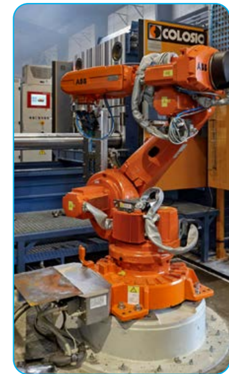
Cycle time could further be decreased to 46 seconds, however, now the limiting factor is the die casting cell robot.
